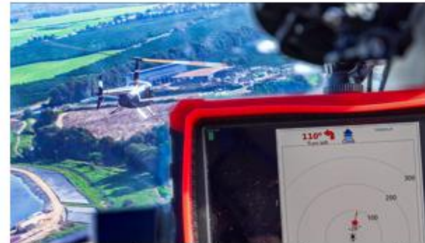
C&CAS onboard 2 helicopters, the rear helicopter's steering command: 'turn left & climb'. Flight test, Dec. 2023, Israel
